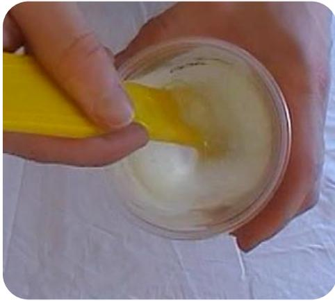
bubbles at their premature stage will conclude with an uneven surface and a finish that is not completely transparent. A number of measures can be taken to counteract and limit bubble formation. Firstly the operator must slowly mix the resin thoroughly with the supplied mixing stick that comes with the MC resin system for 4-5 minutes. This mixing stick contains holes and is especially designed to burst big
