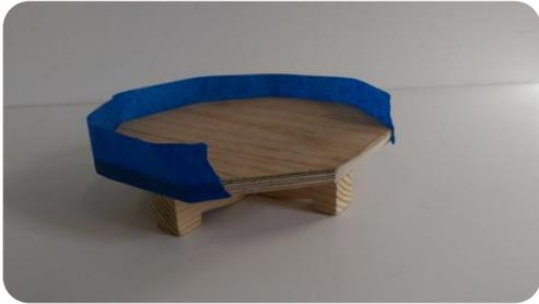
Masking Tape is an extremely useful product when casting resins onto irregular shaped objects. Masking tape is impermeable to epoxy resin and once the curing process is fully completed the tape can be peeled off with comfort leaving the edges of the casting smooth and square. It is notable however that this process is only conventional with a base, namely, the precise shape of the preferred casting.
